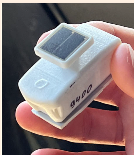
The transmitter is solar powered, weighs 16 grams and will last at least three years. It is mounted on a foam pad and strapped to the bird's back with teflon straps to avoid irritating the bird. The transmitter itself costs $1,500 and requires cell service that is used to send data to an app on Nick's phone.
